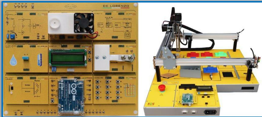
Consisting of simulator and electronic boards, for the study of a semi-automatic warehouse found in industrial environments. They include sensors and actuators so as to develop a complete course on main features of a semi-automatic warehouse and its applications.
