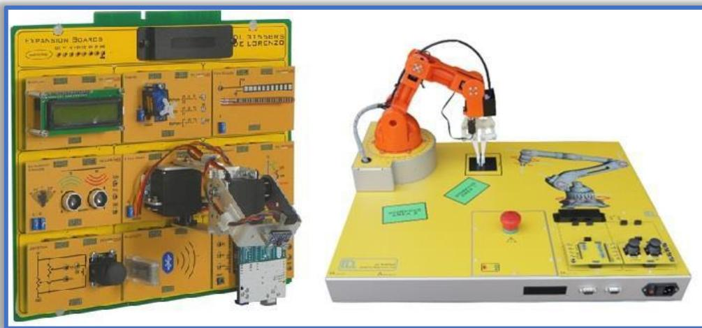
Consisting of simulator and electronic boards, for the study of the properties and control techniques of a 5-axis robotic arm used in industrial environments. They include sensors and actuators so as to develop a complete course on robot control systems. The students can interact with the hardware in a simple way through software explaining step-by-step the operation of the system.
