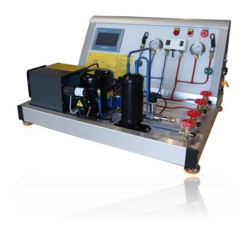
This smart system for the study of refrigeration and air conditioning integrates the most advanced components to control and optimize the systems in an efficient and sustainable way. It uses sensors, transducers, measurement devices and management and supervision software to monitor and collect real-time data on critical parameters such as pressure, humidity, flow and temperature.
