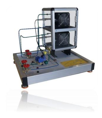
This trainer is designed to show the different modes of variation of temperature and relative humidity in cold rooms to protect the goods being stored from the activity of microorganisms growing at ambient temperature.
