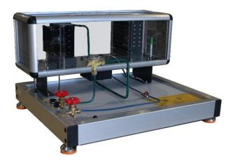
This trainer is designed for the complete and exhaustive study of thermodynamic transformations the air undergoes when crossing a three-section central air-conditioning unit.
