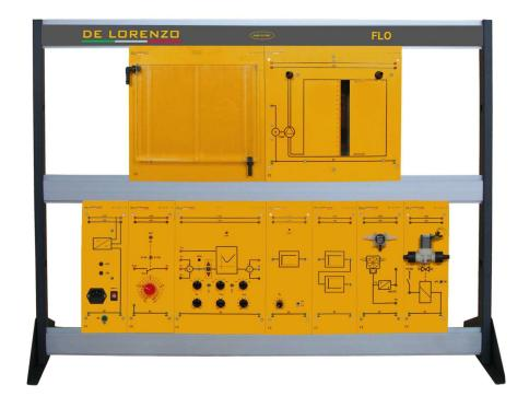
This laboratory must be designed for the study of Flow control application to allow the student a practical training, based on the performance of guided experiments. Industrial type components are educationally adapted by using a modular panel system to permit the step by step assembling from the simplest circuit to the most complex system.
