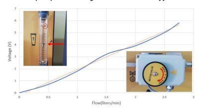
During these experiments, the students learn how to measure the water flow rate by using the engraved scale of the direct flow meter or the turbine flow sensor. After analyzing the results, they must be able to implement the tuning of the PID control of the system with optimum stability.
