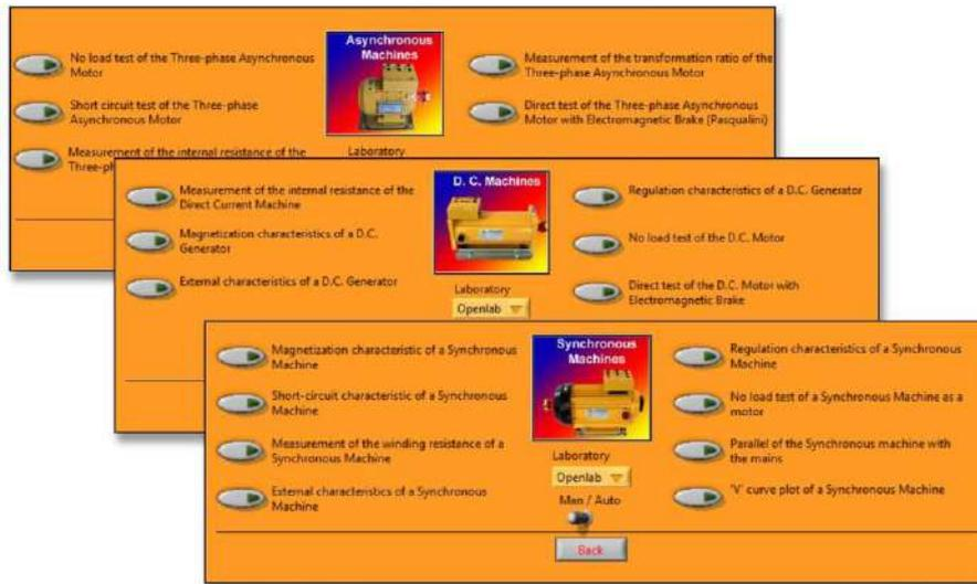
The **DL 8330SW** is a software developed for the acquisition and display the data of the DL OPENLAB\_A laboratory. It is developed in LabVIEW and communicates with the instruments (DL 10065N and DL 10050N) through the data acquisition module (DL 1893) and collect mechanical data (speed and torque) as well as electrical data (AC and DC, Voltage, current and Power).
